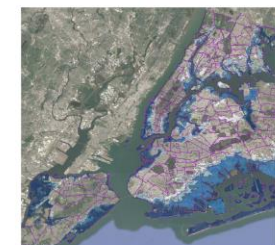
Simulated "Worst-Case" flooding event (blue) in NYC overlaid with Neighborhood Tabulation Area borders (purple), illustrating widespread flood risk. Source: NYC OpenData.
